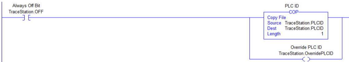
3. The **TraceStation.StationID** setting can be overridden to change the identity of the station, which is typically used to affect permissions downstream, or if multiple models can be run on the machine that have different amounts of process data and need to be separated logically in the database.
