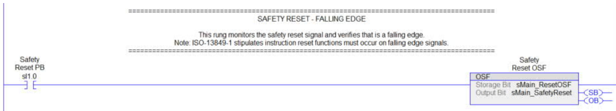
Figure 21: Safety Reset Signal – Falling Edge
