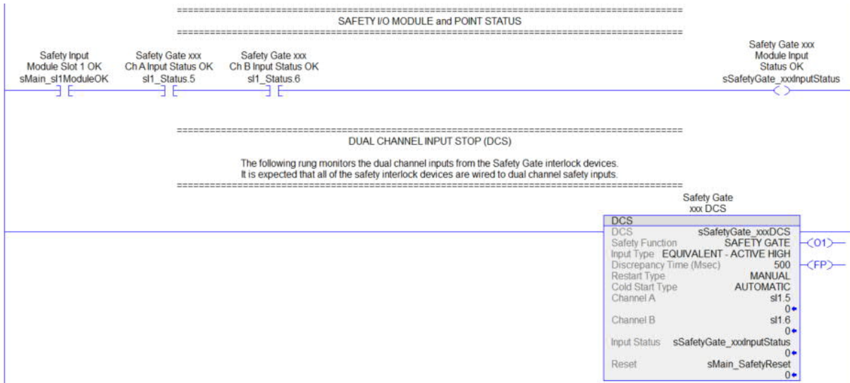
Figure 25: Safety Gate Input Status and DCS Instruction
