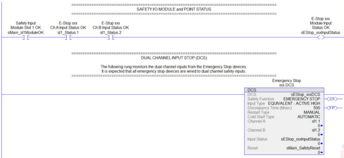
Figure 23: Emergency Stop Input Status and DCS Instruction
