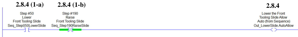
Figure 11: Example Auto Allow Logic (Motion Towards the Work Position)
